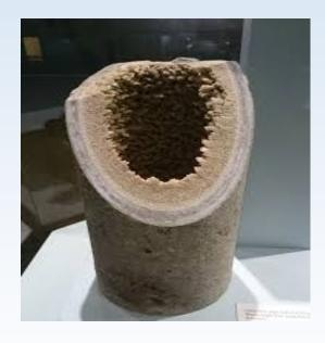
It is estimated that more than 600,000 miles of AC pipe exist in the United States. The life span of AC pipe ranges from 50 to 75 years. Pipe installed during the 1950's and 1960's has reached, or is reaching, the end of its usable life. Wear and tear from intended use and natural erosion results in corrosion and deterioration.
